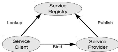
Figure 1. The basic Service Oriented Architecture [5]
